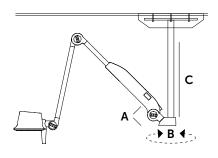
$A = 90^{\circ} (\pm 45^{\circ}) \quad B = 360^{\circ}$ **C** = FROM 250 mm TO 1.100 mm
