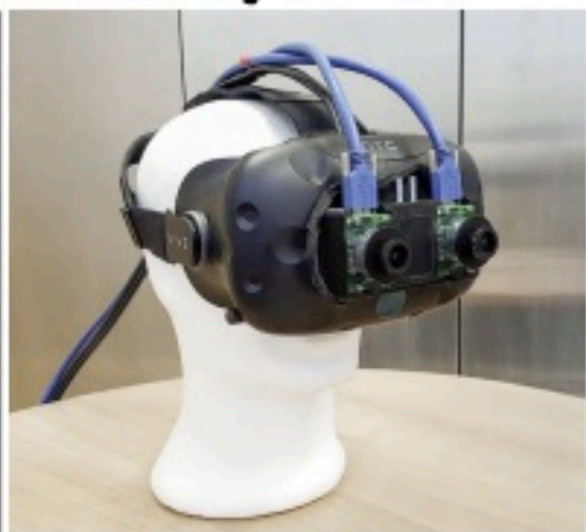
Head-mounted displays used to develop prototypes for medical AR systems. Both head-mounted displays have been developed in Munich – but are not conceived for use in the operating theatre (too many cables, too heavy)
