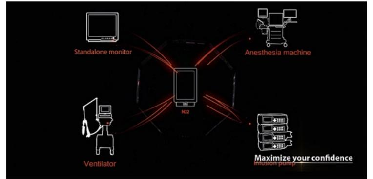
The BeneLink Interfacing Module integrates monitored data from other bedside devices
